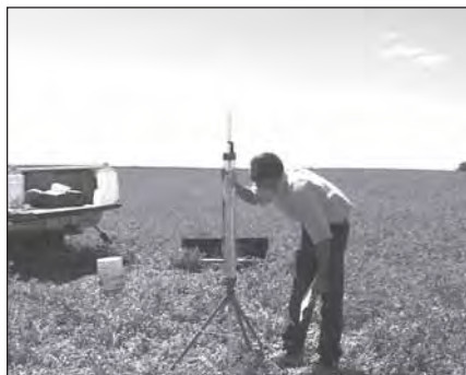
To measure the saturated hydraulic conductivity of the soil, I use a Guelph Permeameter.
