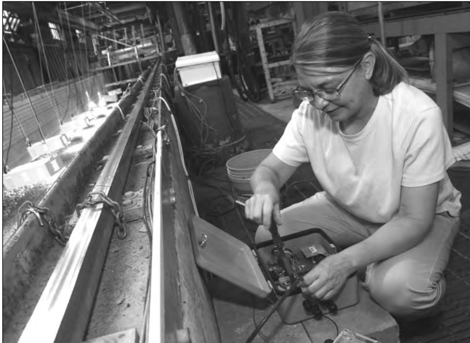
NCED post-doc Nancy Brown works in the Main Channel facility to determine effects of algal growth on sediment transport during flood periods.
