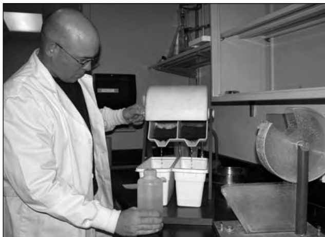
Dan Breneman demonstrates the usefulness of his lab’s new and improved water sample splitter. The original splitter is in the foreground.
