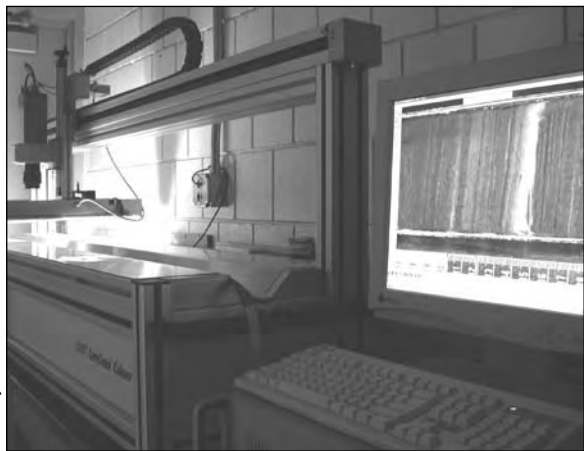
LacCore's linescan camera produces digital core images at a resolution of 10 pixels per millimeter.
