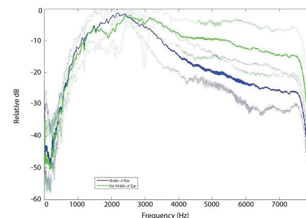
The solid blue line in this figure correlates to the response of the middle of the tympanum. The solid green line corresponds to the response of the outer tympanum. The amplitude of the frequency response is normalized to its peak value (so the highest value = 0). The dotted lines blue and green correspond to the highest and lowest response of the inner and outer tympanum respectively.
