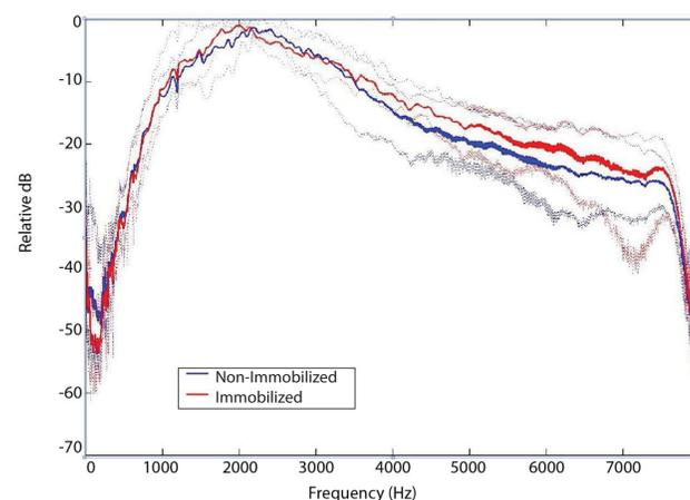
The solid blue line in this figure correlates to the response of the non-immobilized frogs (n=7). The solid red line corresponds to the immobilized frogs (n=7). The amplitude of the frequency response is normalized to its peak value (so the highest value = 0). The dotted lines blue and red correspond to the highest and lowest response of the non-immobilized and paralyzed frogs respectively.
