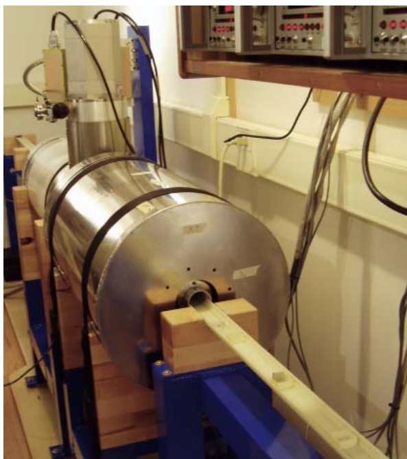
Figure 1. The new magnetometer. Visible from right to left are a portion of the sample handling track, the degausser/ARM unit, and the measurement region with pulse-tube cryo-cooler.
