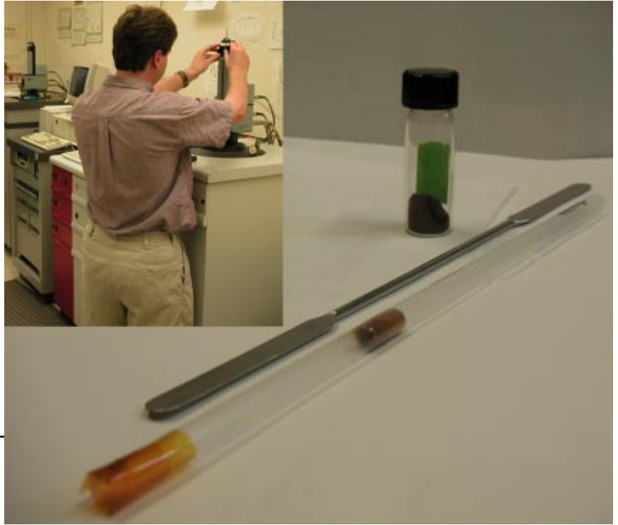
Yohan Guyodo loading a sample of As-substituted ferrihydrate in his favorite IRM instrument, the magnetic properties measurement system (MPMS).
