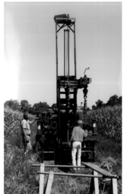
Mobile hollow stem augur at work at Pittsburg Basin. Jeff Dorale and Jim Neal coring site PBAS 94-5a.
