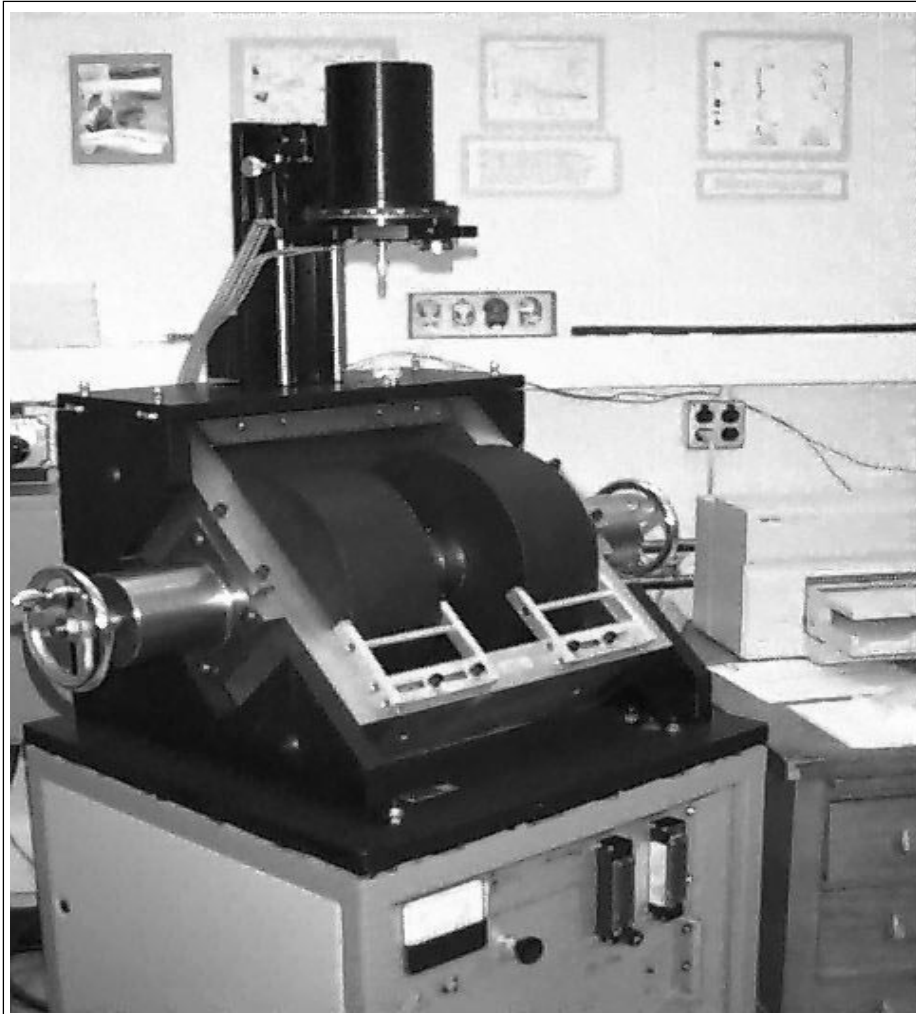
The new Vibrating Sample Magnetometer (VSM) from Princeton Measurements Corporation enables measurement of magnetization as a function of applied field (to 1.8 T), temperature (to 750 C) and orientation.
