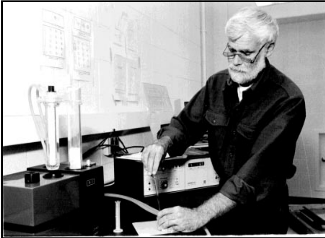
Jim Marvin poses in front of the Kappabridge while loading a powdered sample for thermomagnetic analysis.
