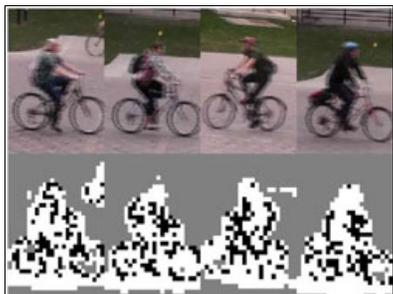
The system converts video data into small image "patches" and classifies each patch as a bicycle (black) or pedestrian (white) before making an overall classification of the entire object.
