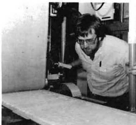
Kaufert Laboratory houses a small scale paper machine where the students learn the basics of papermaking through hands-on experience. Above, Kurt Olsen inspects pulp being fed onto the pilot machine while Tom Edgren (below) monitors the dryer section.
