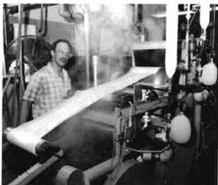
Kaufert Laboratory houses a small scale paper machine where the students learn the basics of papermaking through hands-on experience. Above, Kurt Olsen inspects pulp being fed onto the pilot machine while Tom Edgren (below) monitors the dryer section.
