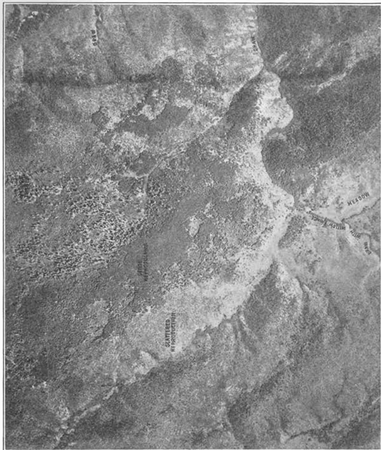
A vertical aerial photo for forest mapping. Taken about 10,000 feet above terrain, scale about 6 inches to 1 mile. Forest types and age classes can be mapped from this in detail.
