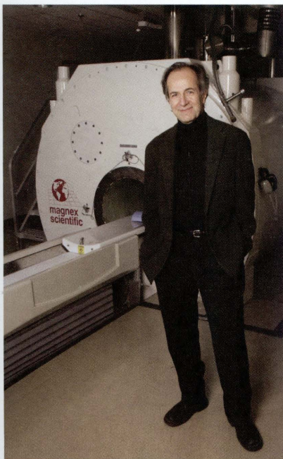
Kamil Ugurbil, Ph.D., will be researching the brain and schizophrenia using this state-of-the-art 9.4 Tesla magnet. Typical hospital magnetic resonance scanners use a field strength of 1.5 Tesla.
