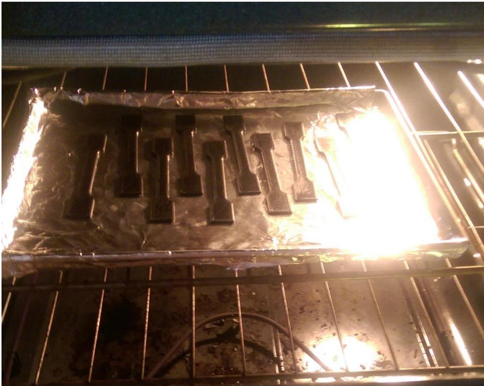
The annealing process was carried out in an electric home oven. For this experiment, two temperatures (185 and 200F) and three lengths of time (10, 30, and 60 minutes) were chosen for the ABS samples. Due to the lower melt temperature of PLA, only one temperature was used (170F) with the same three time intervals used for the ABS samples. For each set, ten samples were tested, all going through the
