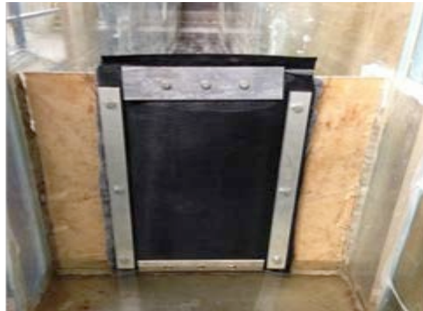
Figure 24. Photograph of the steel wool filter installed in the flume for the pilot-scale study.
