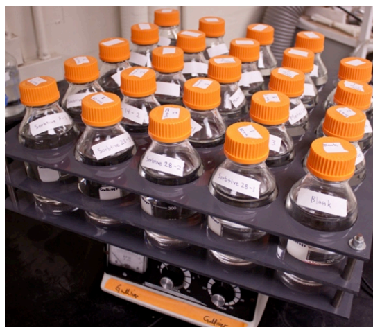
Figure 20. Photograph showing sample bottles set up on a shaker table during the batch study experiments.
