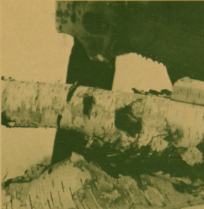
Figure 6. Saw pinching can be avoided by determining where tension and compression occur along the stem and making the final cut on the tension or "opening" side.
