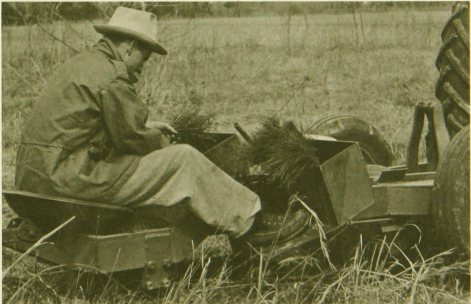
Figure 3. Self-contained system on planter regulates depth of planting.
