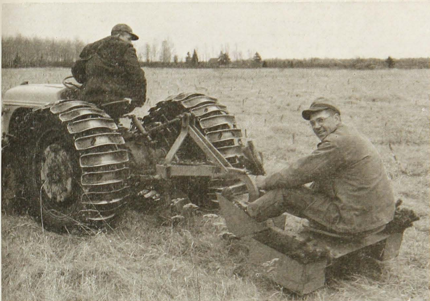
Figure B. Three point hydraulic lift controls planting depth.
