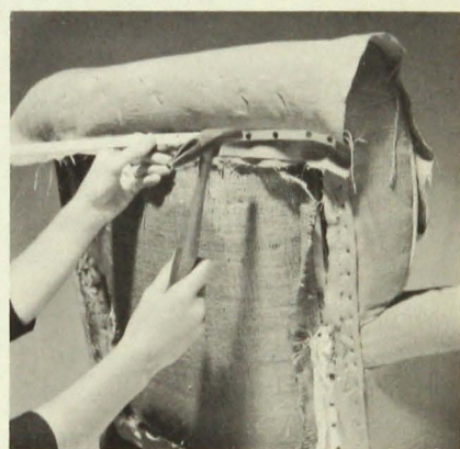
Fig. 53—Blind tacking outside back at top.
