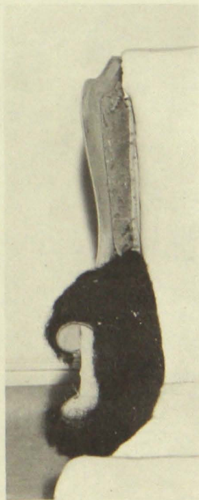
Fig. 33—Stitch padding to burlap on inside arm.
