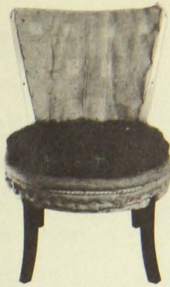
Fig. 57 —Moss padding sewed in place. Seat ready for cotton padding. Back webbing covered with burlap.
