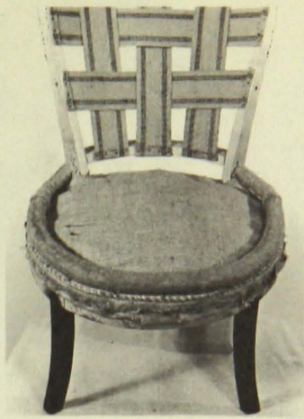
Fig. 56 —The fireside chair. Webbing and springs in place, covered with burlap and hard edge roll put on.
