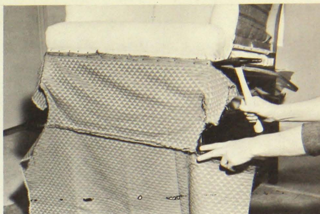
Fig. 43—Blind tack front seat edge.
