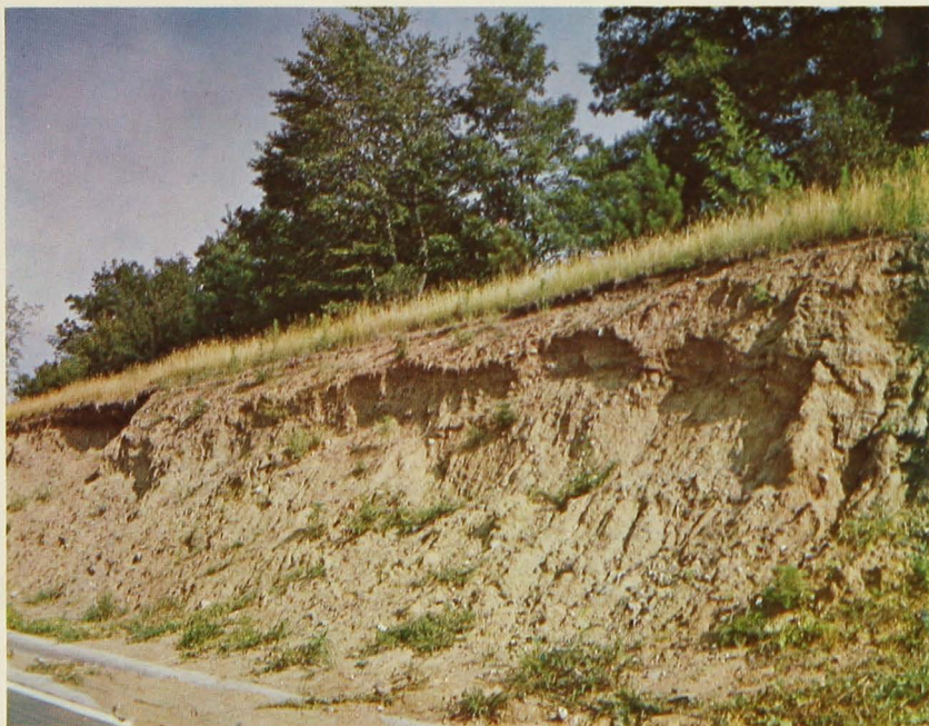
Figure 25. Profile of red till near Highway 36 in Ramsey County. The soil developed here is Group 4, Milaca sandy loam.
