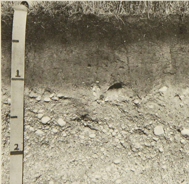
Figure 19. Profile typical of Group 2 soils shows medium-textured material above and sandy and gravelly material below. Depth of the horizons varies within the group. Depth in feet is indicated.
