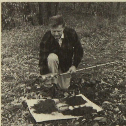
A soil auger is used to make a site evaluation.
