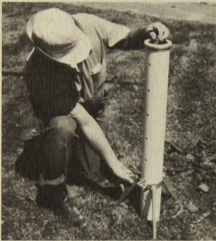
The percometer sets vertically with the adjustable tripod.
