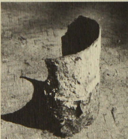
Metal septic tank baffles corrode easily. Avoid using them.
