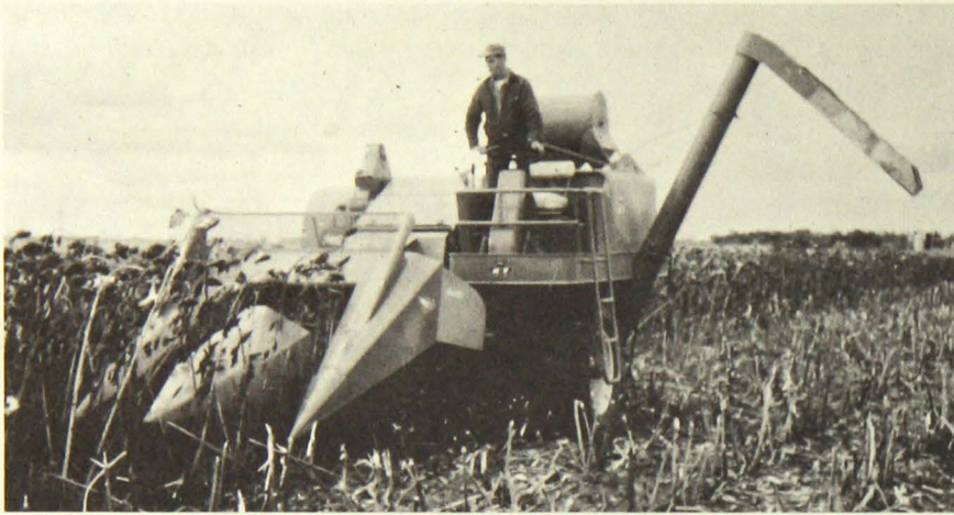
Figure 14. A combine with a corn head attachment can be used if acreage is too small to warrant purchase of a sunflower header. Shattering seed will be lost because there are no pans to catch it.
