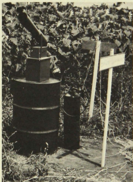
Figure 28. A welder's tank supplies acetylene gas for this bird frightener. The gas is ignited by a glow plug powered by a storage battery. The explosions, which come at 45-second or longer intervals, are several times louder than a shotgun.
