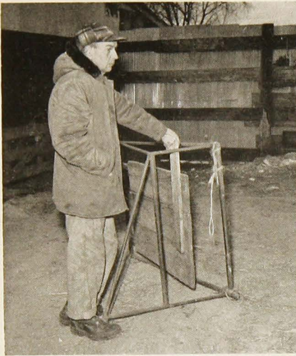
Fig. 7. This portable dodge gate, farm-built, speeds up "topping out" lambs that are already fat enough for market.
