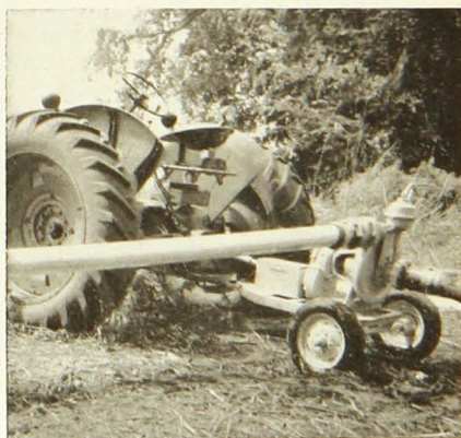
Fig. 18. Pumping for irrigation from power take-off of tractor.
