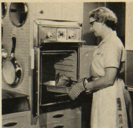
Fig. 6. The bottom of the inside of this oven is 32 inches from the floor. (Beltsville Energy-Saving Kitchen, USDA, 1956.)
