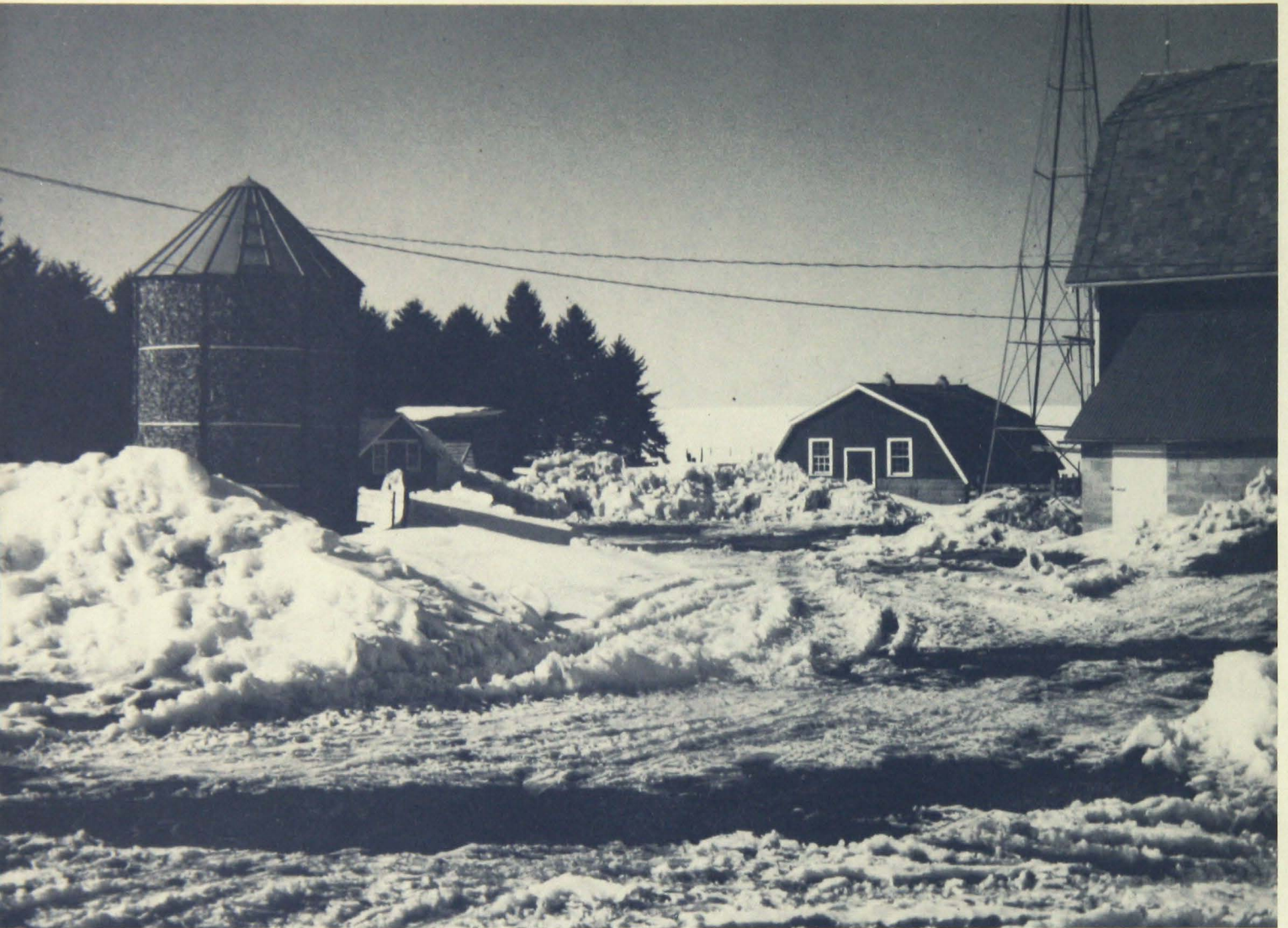
Figure 2. Shelterbelt too close to the farm buildings. Snow dumps into the farmstead area. Energy in the form of tractor fuel and hand labor is required in snowplowing and shoveling to clear work area for performing daily chores.
