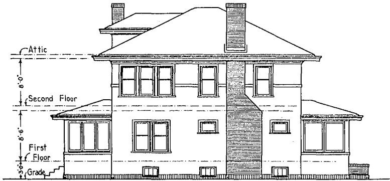
Plan 124. Elevation of hip-roof farmhouse, Plan 122
