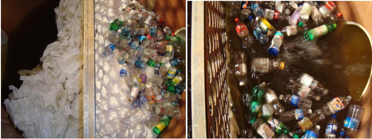
**Figure 3-10: (Left) loading phase of Test 1. (Right) washout phase of Test 1. The flow is from right to left.**
