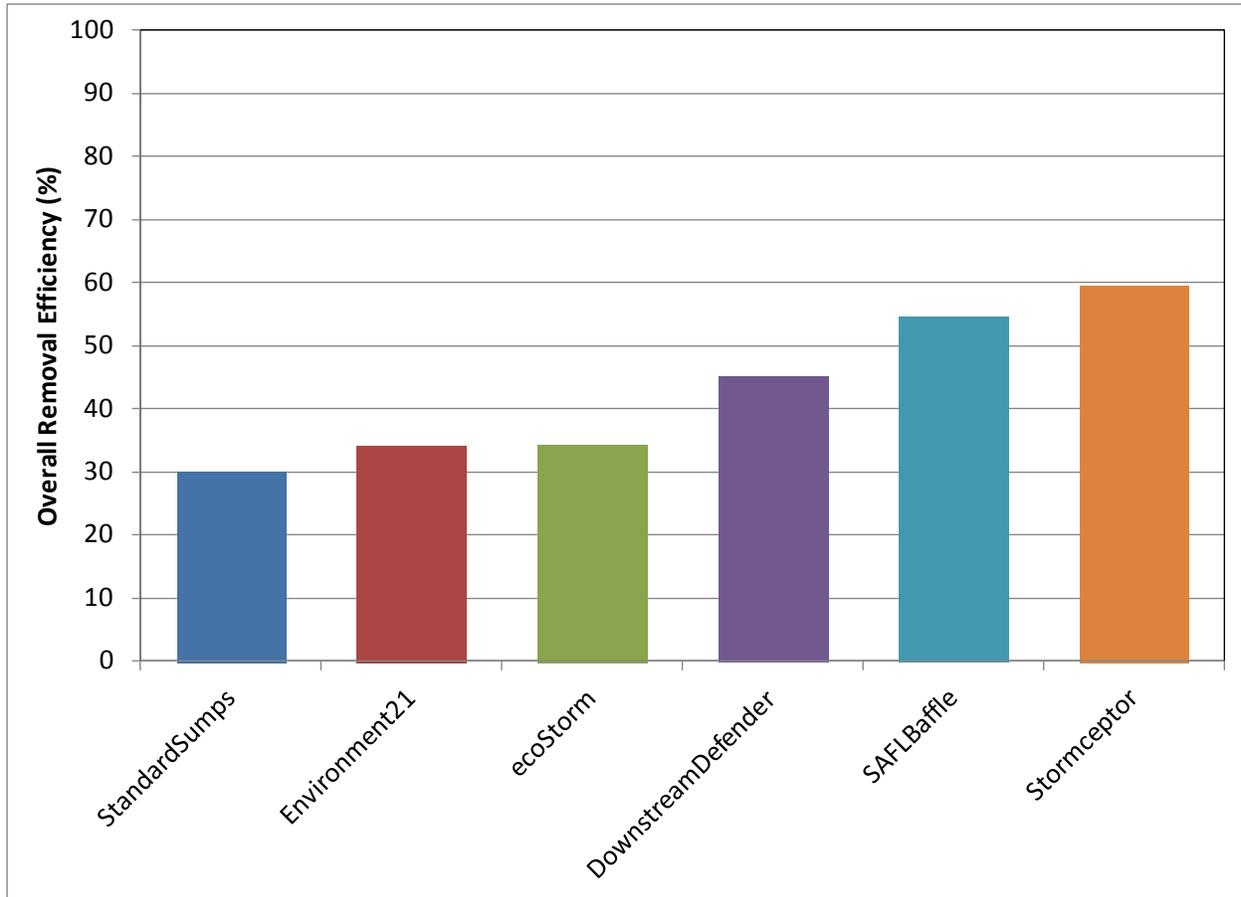
**Figure 7-1: Overall removal efficiencies of ecoStorm, Downstream Defender, Environment 21, Stormceptor, Standard Sumps, and Standard Sumps equipped with a SAFL Baffle in removing OK110 from stormwater runoff of a 5-acre watershed in Minneapolis, MN, area.**
