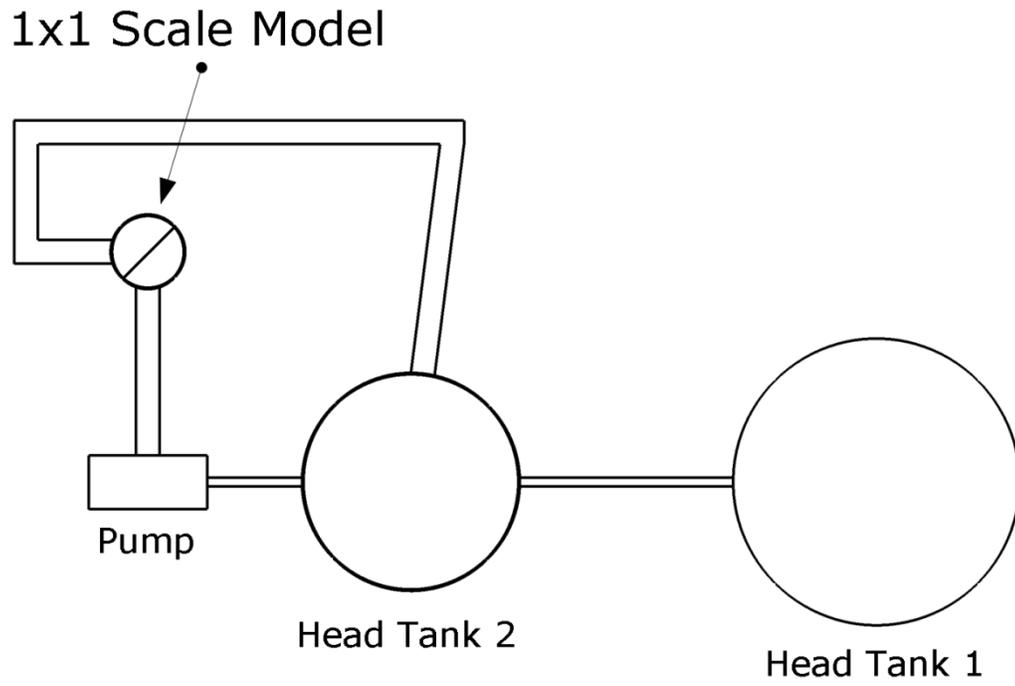
**Figure A-12: A plan view of the 1x1-90 degree outlet sump setup.**
