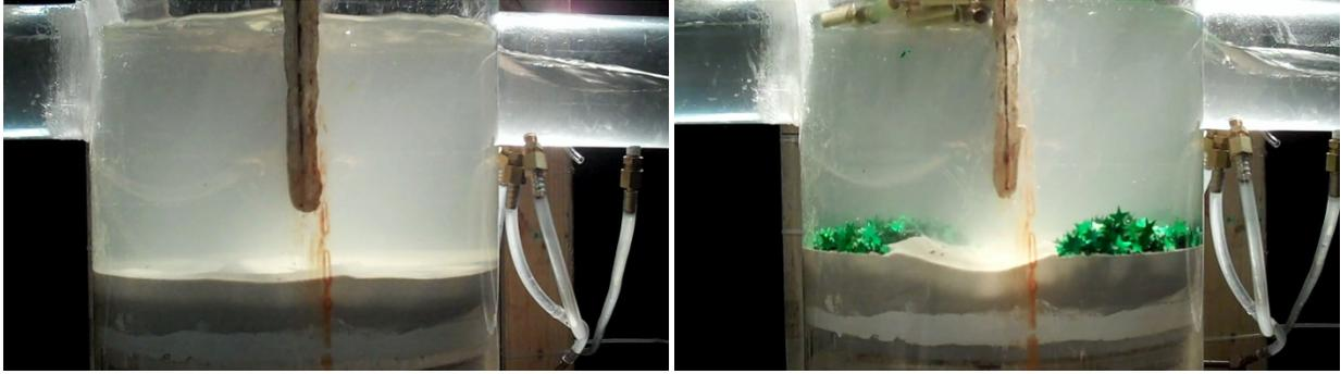
**Figure 3-8: The final seconds of washout Tests 2 and 3 on the 1×0.5 model. Water is flowing from left to right.**
