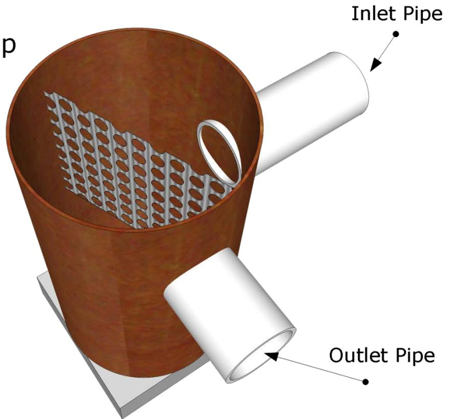
Figure A-8: The 6×6-90 degree outlet sump setup.
