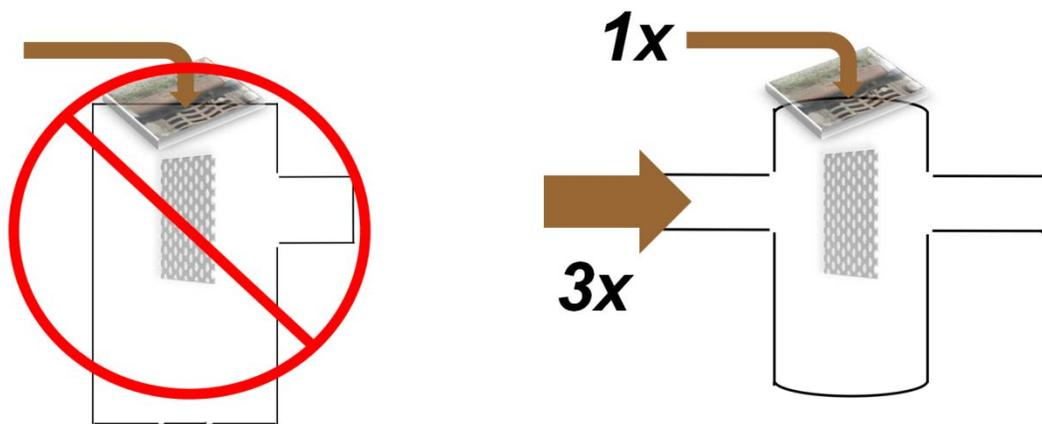
**Figure 8-1: (Left) inlet grate flows into sump manholes cause washout and decrease removal efficiency of the device. (Right) install SAFL Baffles in sumps where the catchment feeding the inlet pipe is three times the size of the catchment feeding the inlet grate.**
