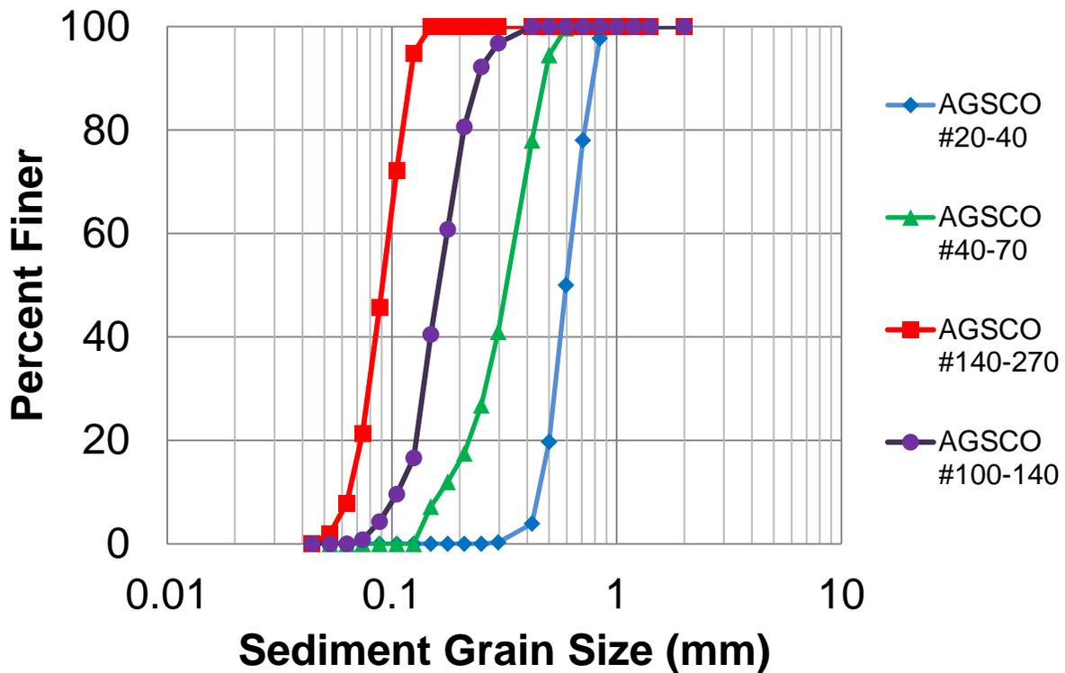
Figure C-1: Sediment grain sizes for four AGSCO products.
