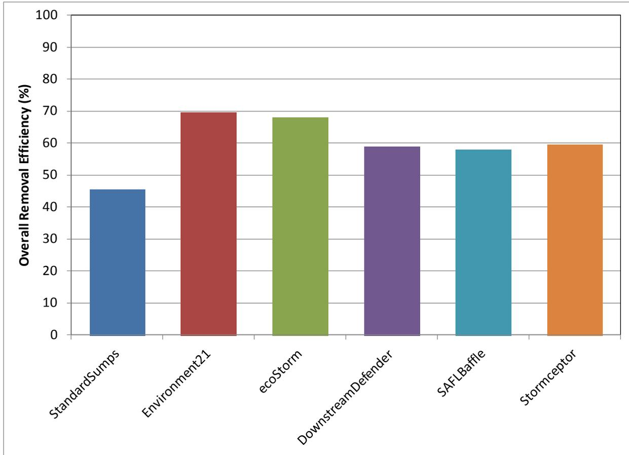
**Figure 7-2: Overall removal efficiencies of ecoStorm, Downstream Defender, Environment 21, Stormceptor, Standard Sumps, and Standard Sumps equipped with a SAFL Baffle in removing OK110 from stormwater runoff of a 5-acre watershed in Minneapolis, MN, area by diverting flows larger than 1 cfs (except for Stormceptor which is equipped with an internal bypass).**
