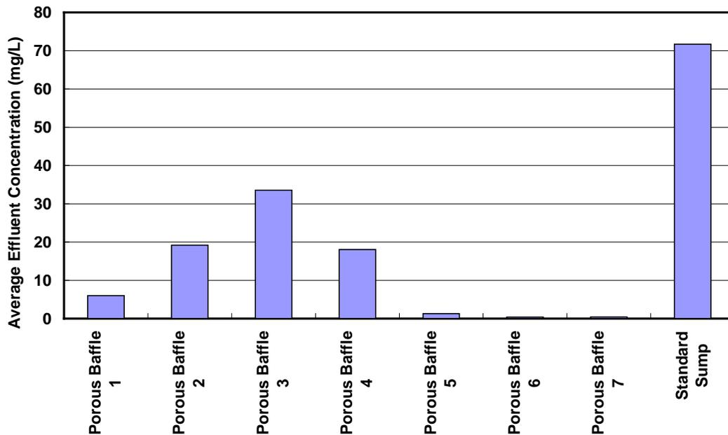
**Figure 2-3: Scale model porous baffle washout results.**
