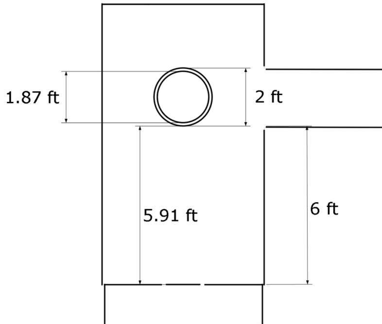
**Figure A-10: A section view of the 6×6-90 degree outlet sump setup. The sump rests on a square wooden platform.**
