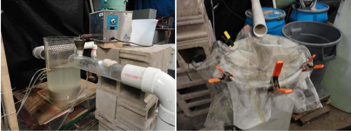
**Figure A-6: Scale model testing system. (Left) water travels from right to left through the sump. (Right) water exits the sump through a PVC pipe system and travels into a head tank protected by a mesh screen and 0.00079-in (20  $\mu\text{m}$ ) filter.**
