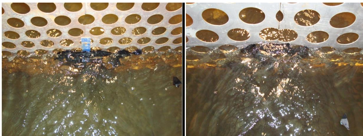
**Figure 3-16: (Left) the clogging pattern for vinyl leaves on the 3-inch (7.6 cm) hole diameter SAFL Baffle and (right) on the 5-inch (12.7 cm) hole diameter SAFL Baffle. These views are from above the inlet pipe, looking downstream.**
