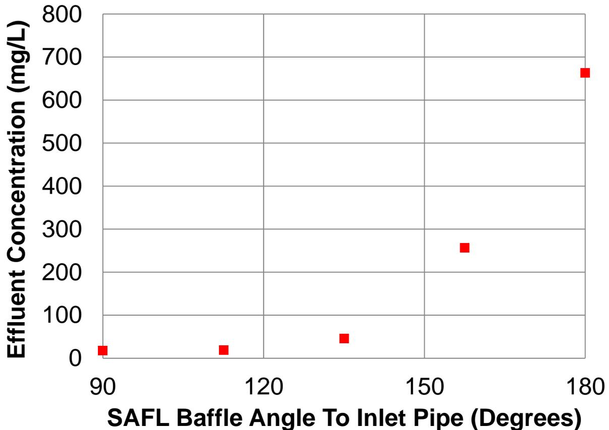
Figure 4-4: 1×1-90 degree outlet washout testing summary.
