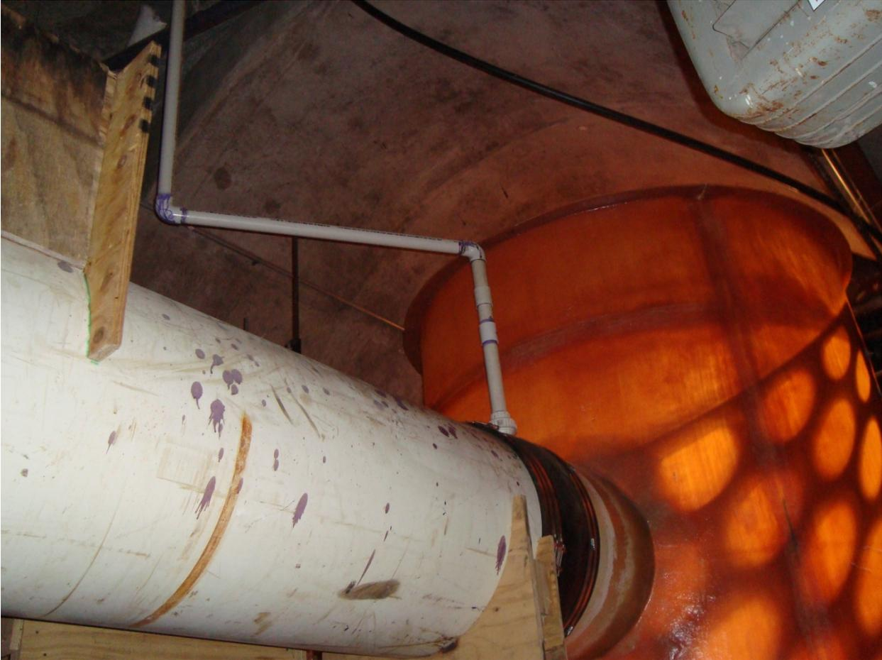
**Figure 2-7: A view of the slurry pipe used to feed sediment into the sump.**
