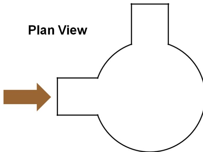
**Figure 1-3: A 90 degree outlet sump manhole.**
