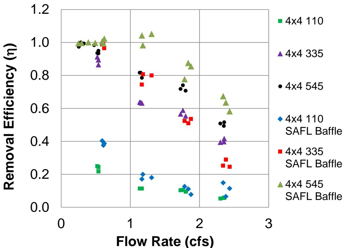
Figure 2-10: The 4×4 ft sump performance results with and without the SAFL Baffle.
