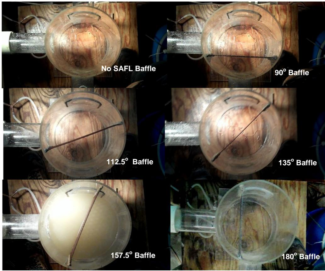
**Figure 4-2: Plan views of 1×1-90 degree outlet washout testing configurations: no baffle, SAFL Baffle oriented at 90 degrees, 112.5 degrees, 135 degrees, 157.5 degrees, and 180 degrees. Water enters the sump from the bottom of picture and leaves from the left.**
