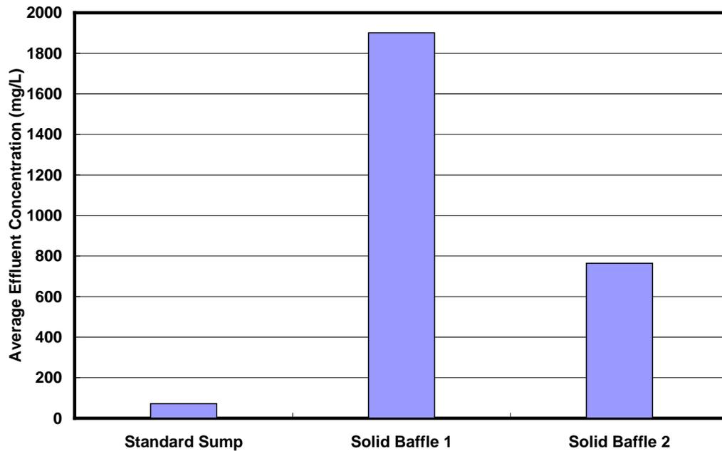
**Figure 2-2: Scale model solid baffle washout results.**
