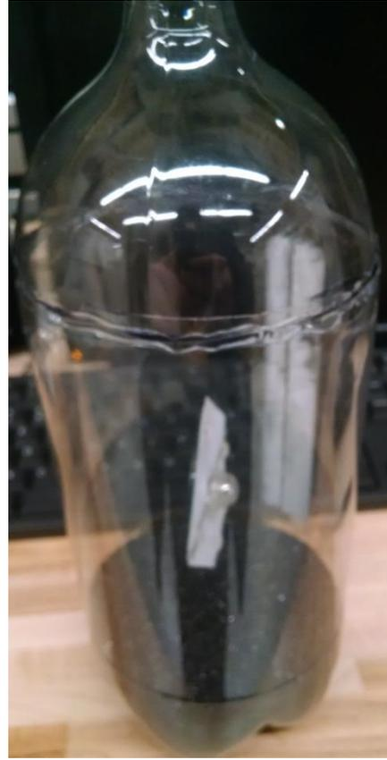
Figure 3 (above left) shows a front view of the bottle, with the mirror hanging approximately in the middle, and some sand in the bottom as a weight to hold the bottle down such that it isn't disturbed by local vibrations.
