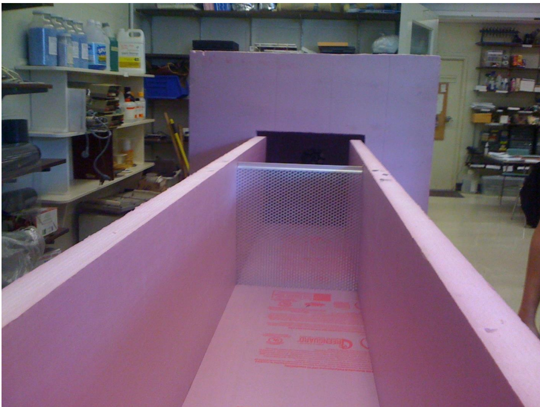
Fig. 5. Interior of the wind tunnel with a perforated plate in place as seen through the open top.
