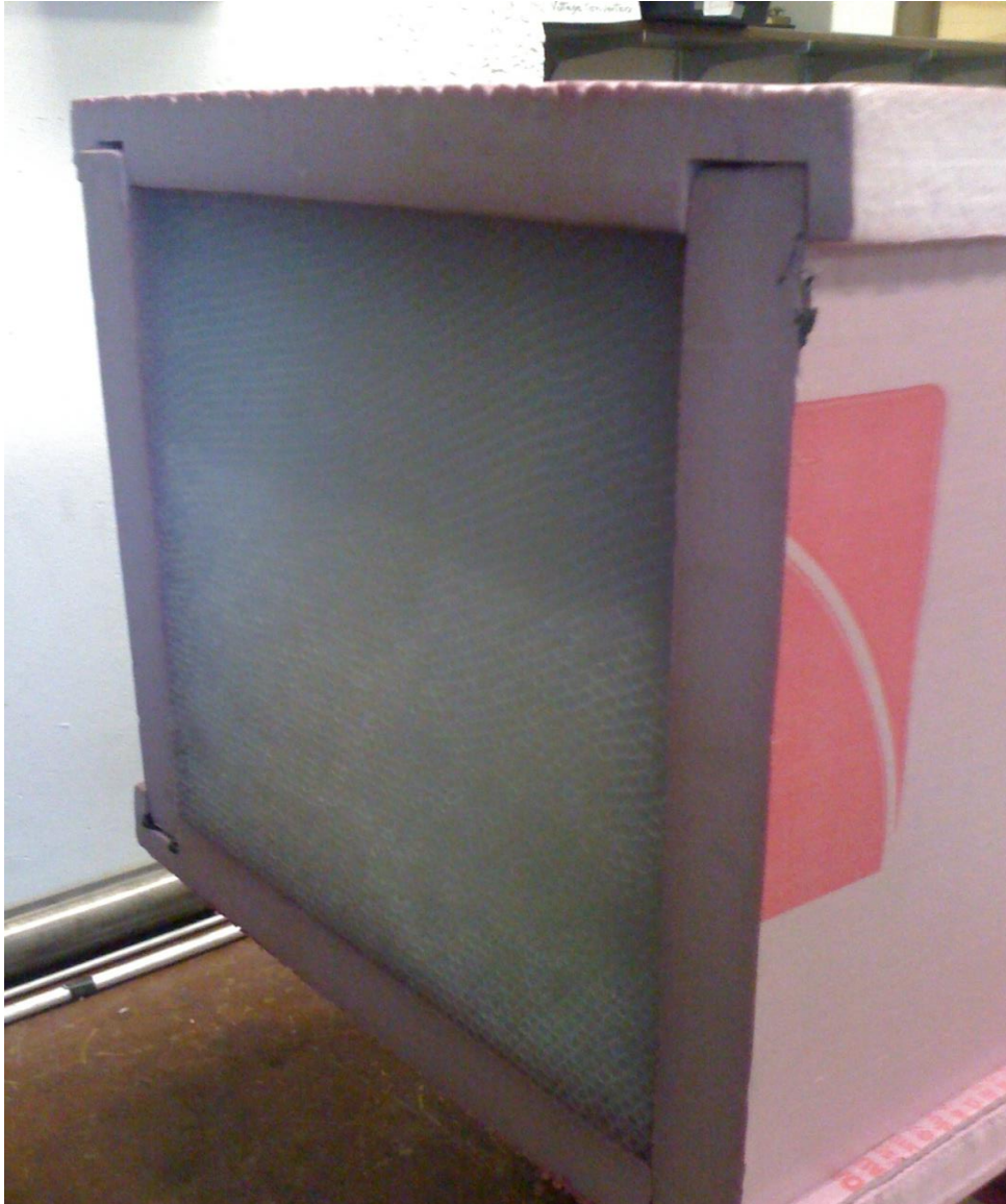
Fig. 4. Inlet to the wind tunnel showing the flow-straightening section.
