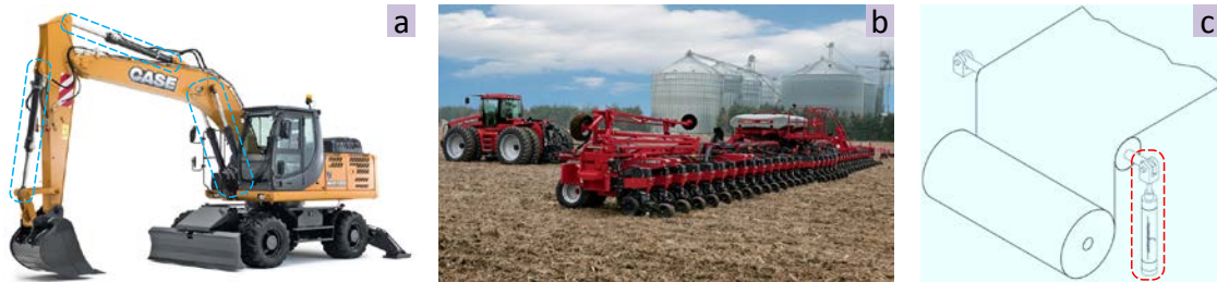
Figure 3-1. Potential applications of piston position estimation in (a) hydraulic cylinders of an excavator for automatic excavation, (b) hydraulic cylinders of a planter for maintaining optimal seeding depth, and (c) a pneumatic actuator for web guide. Photos are courtesy CNH® and Bimba®.
