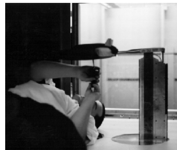
Installing Aerocar in Wind Tunnel, Travis Smieja
