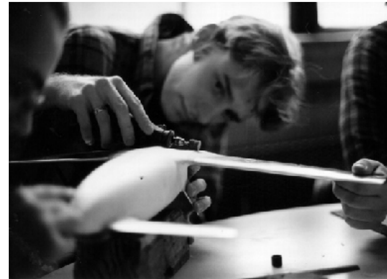
AEM Senior Chris Mitchel preparing Reusable Launch Vehicle model for testing in the wind tunnel.
