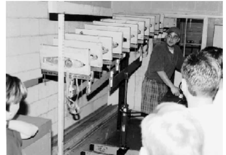
Load Testing of Wing
