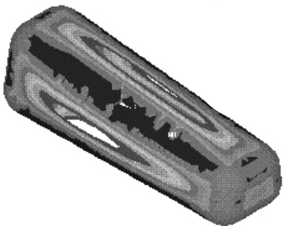
ANSYS Solution of Fall Quarter Liquid Oxygen Tank with 1.0 Inch Skin Thickness
