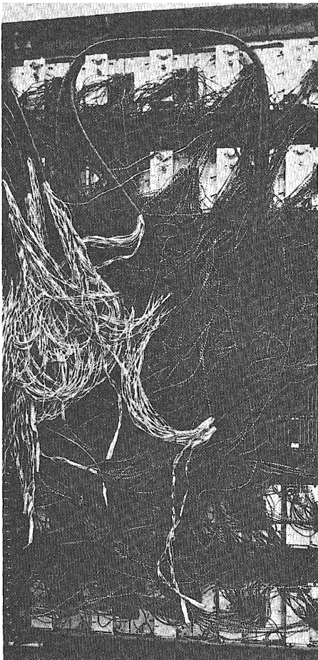
Behind the "mainframe" of the CDC 6600, the wire scheme is without pattern to prevent "parity errors" caused by the alignment of magnetic and electric fields.
