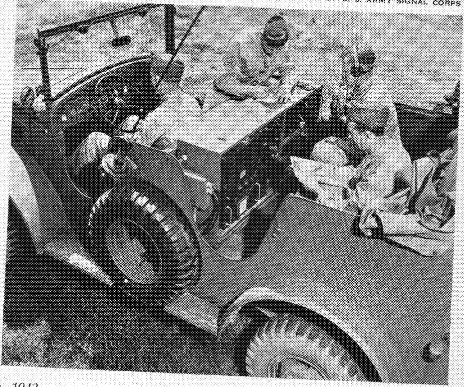
THE RADIO SHOWN is protectively mounted to prevent damage from shock. The set is equipped to receive and send both code and voice over short-wave bands.
