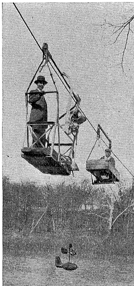
Modern stream gaging car, showing a self-reading depth recording drum.
