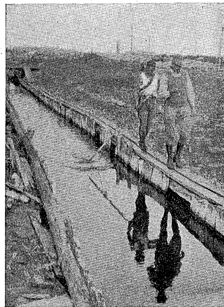
Meter rating at Cass Lake. The meter is towed by hand through still water.
