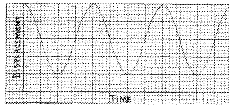
FIG. 2. TIME-DISPLACEMENT CURVE FOR FREE SINUSOIDAL VIBRATIONS.
