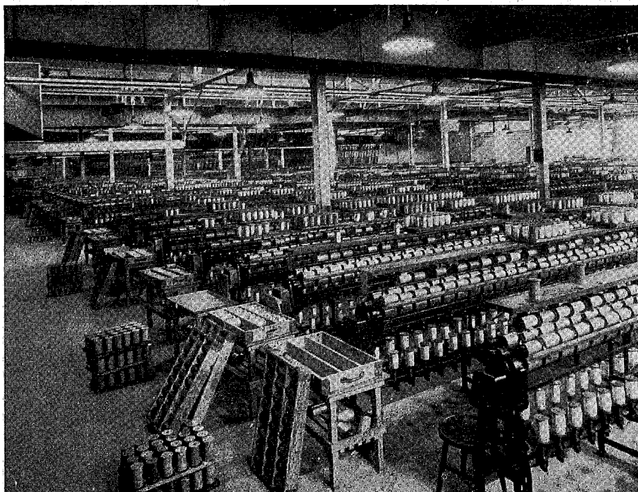
This cut illustrates the throwing operation which consists in putting the twist in the yarn by winding it from one spool to another. One of the spools is driven at a high rate of speed while the other turns very slowly.
