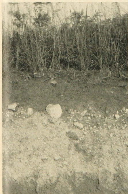
FIG. 10. Typical profile of a prairie soil in the Kittson-Peat area
