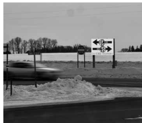
The CICAS-SSA system warns drivers of oncoming traffic at rural unsignalized through-stop intersections.
