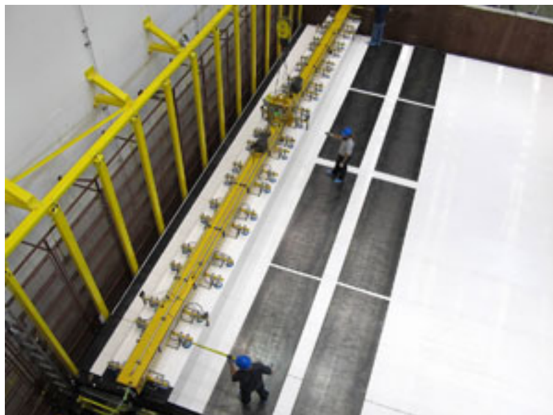
Technicians add modules to the first block of the NOvA detector. Photo by Ron Williams, NOvA lead foreman.
