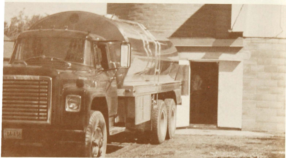
Tandem axle bulk trucks have load capacities of about 3,250 gallons.
