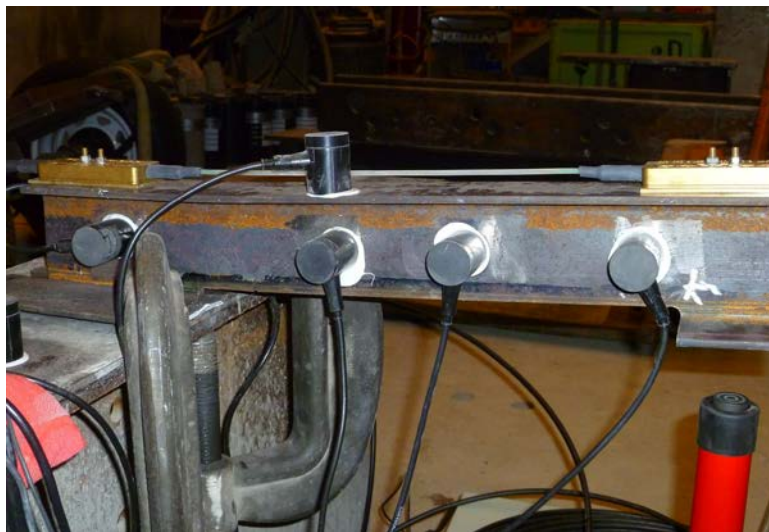
Figure 5.5: Placement of fiber optic sensor on top flange
