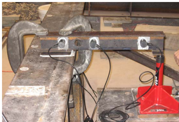
Figure 5.2: Test setup for the second notched beam test
