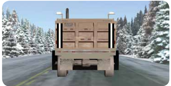
The recommended design features vertical bars of light flanked by dense black material to maximize contrast with the plow's paint.
