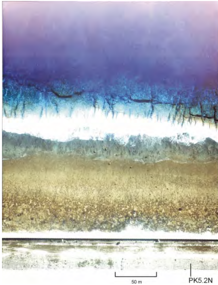
Figure 1.10 Aerial photograph showing underwater extension fractures of the order of 2-m width in the vicinity of PK5N, Irène section (part of the aircraft runway strip, with protective wall, runs parallel to the bottom of the photograph; this region is outside test area 1) [photo courtesy of DIRCEN/CEA]
