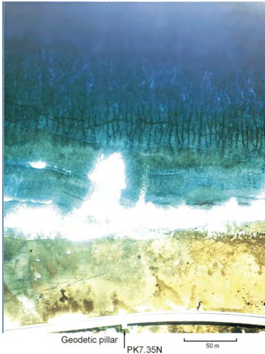
Figure 1.13 Aerial photograph showing extension fractures generated by continuous creep deformation in the ocean slope of the northeastern rim of Mururoa in the vicinity of PK7.4N (Camélia zone), test area 1 (see frontispiece map of Mururoa; several relatively narrow (10 cm ~ 20 cm) fractures (trending ENE) are visible on shore; larger fractures probably up to 2-m aperture, can be discerned under the deeper water) [photo courtesy of DIRCEN/CEA]
