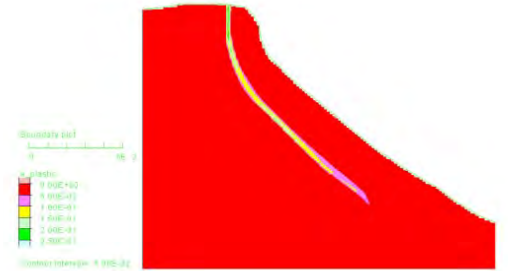
Figure 5.21 Slope in the northern zone, softening model — contours of plastic shear strain for a safety factor \Phi = 2.0
