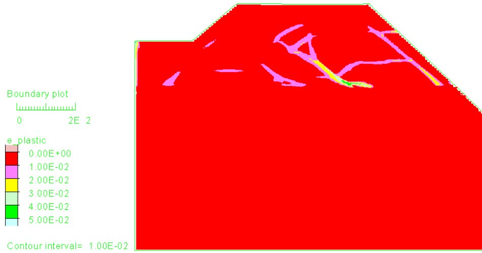
Figure 4.11 Contours of plastic shear strain after a 150-kt explosion
