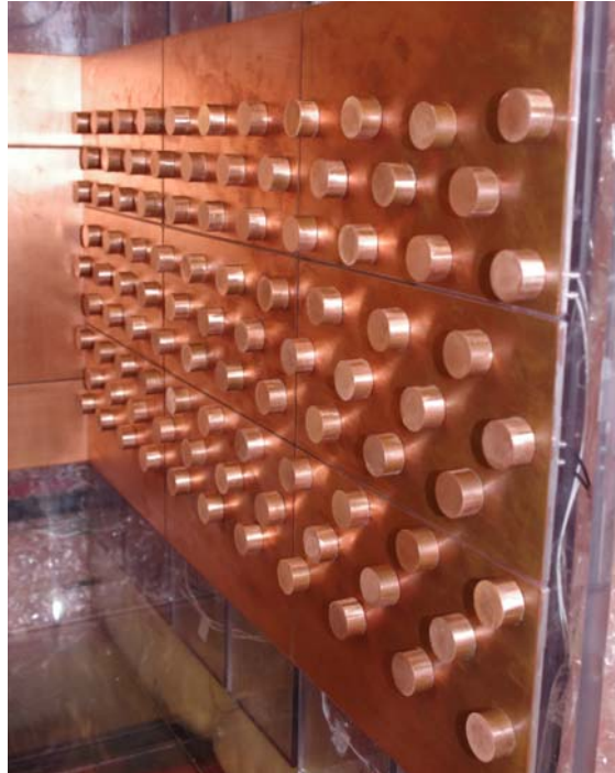
Figure 4.1: Staggered arrangement of pin fins on channel wall for heat transfer measurements
