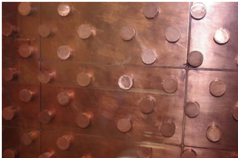
Figure 4.2: Arrangement of pin fins on channel wall for velocity measurements
