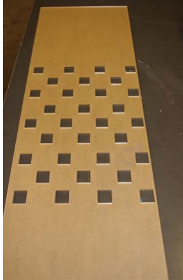
Figure 2.9: Template used to attach copper pieces on the fin wall
