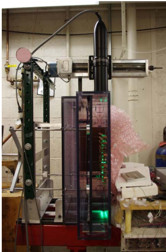
Figure 4.4: Laser probe arrangement on channel wall augmented with pin fins
