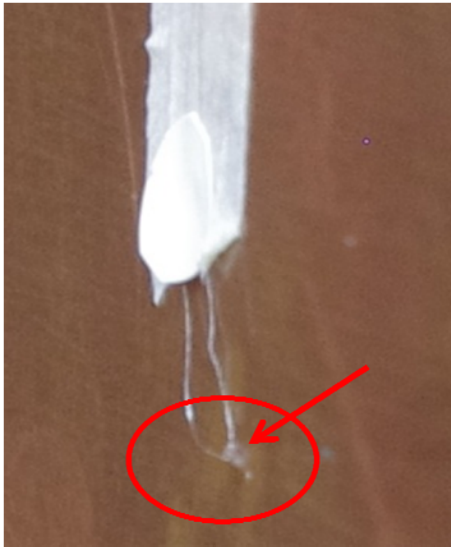
Figure 2.6: Thermocouple mounted on copper plate with a small dab of glue
