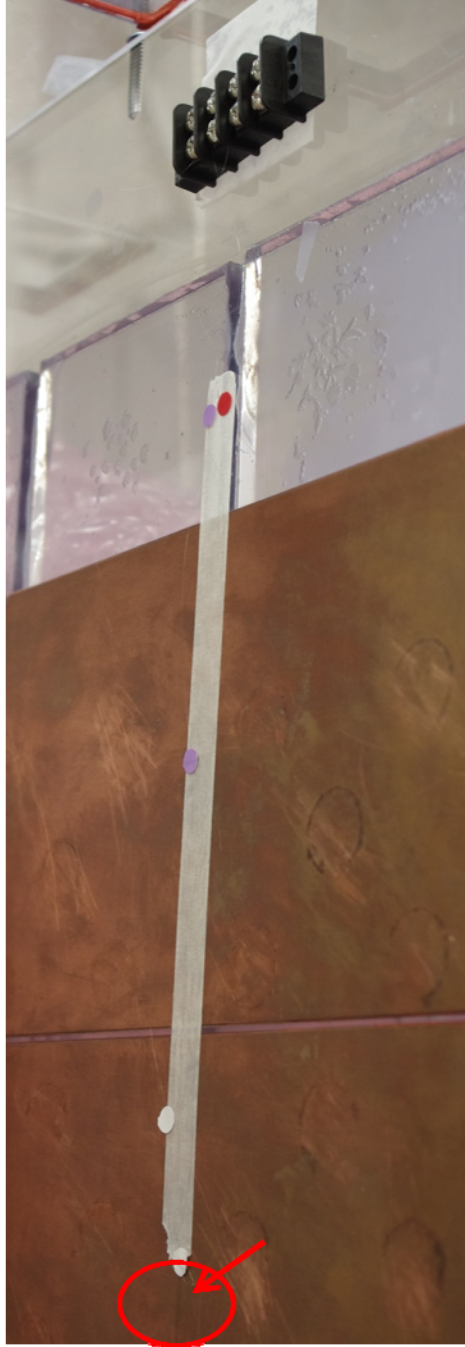
Figure 2.7: Thermocouple mounted on copper plate with a small dab of glue. The thermocouple is then connected to a thicker gauge thermocouple of 76\ \mu\text{m} (0.003 inch) diameter of the same type (top of figure), to transfer the emf as measured by the smaller gauge thermocouple
