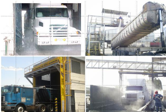
Truck and Equipment washing to control dusts transported outside the plant
