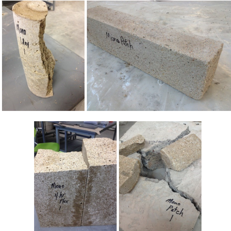
Figure 36: Mono Patch compressive, freeze-thaw, flexural and pull out specimens
