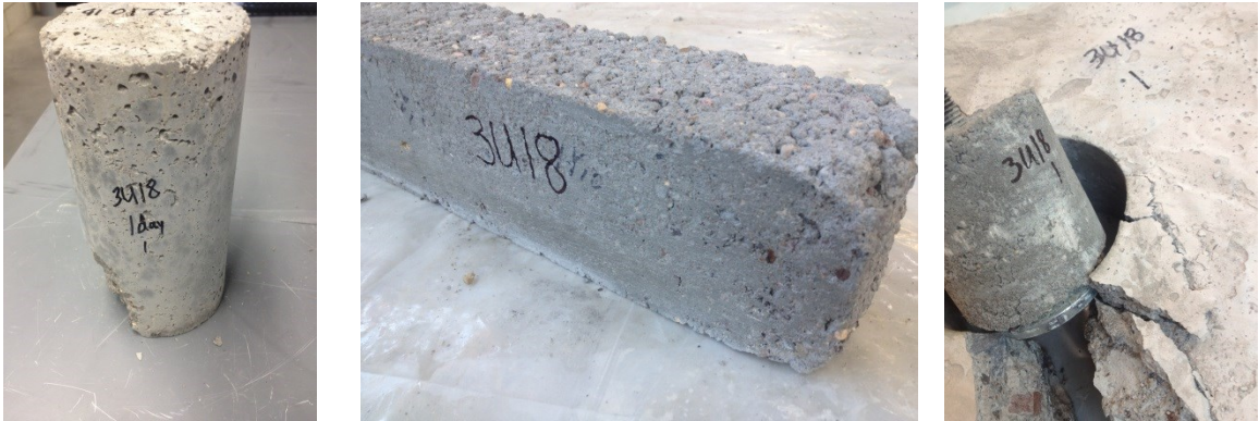
Figure 28: 3U18 compression, freeze thaw and pull out specimens
