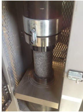
Figure 4: Compression Test Setup
