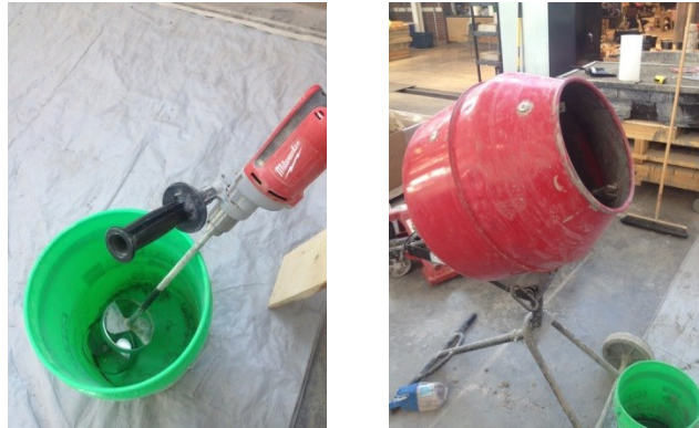
Figure 16: Drill and paddle with a bucket and a standard concrete mixer
