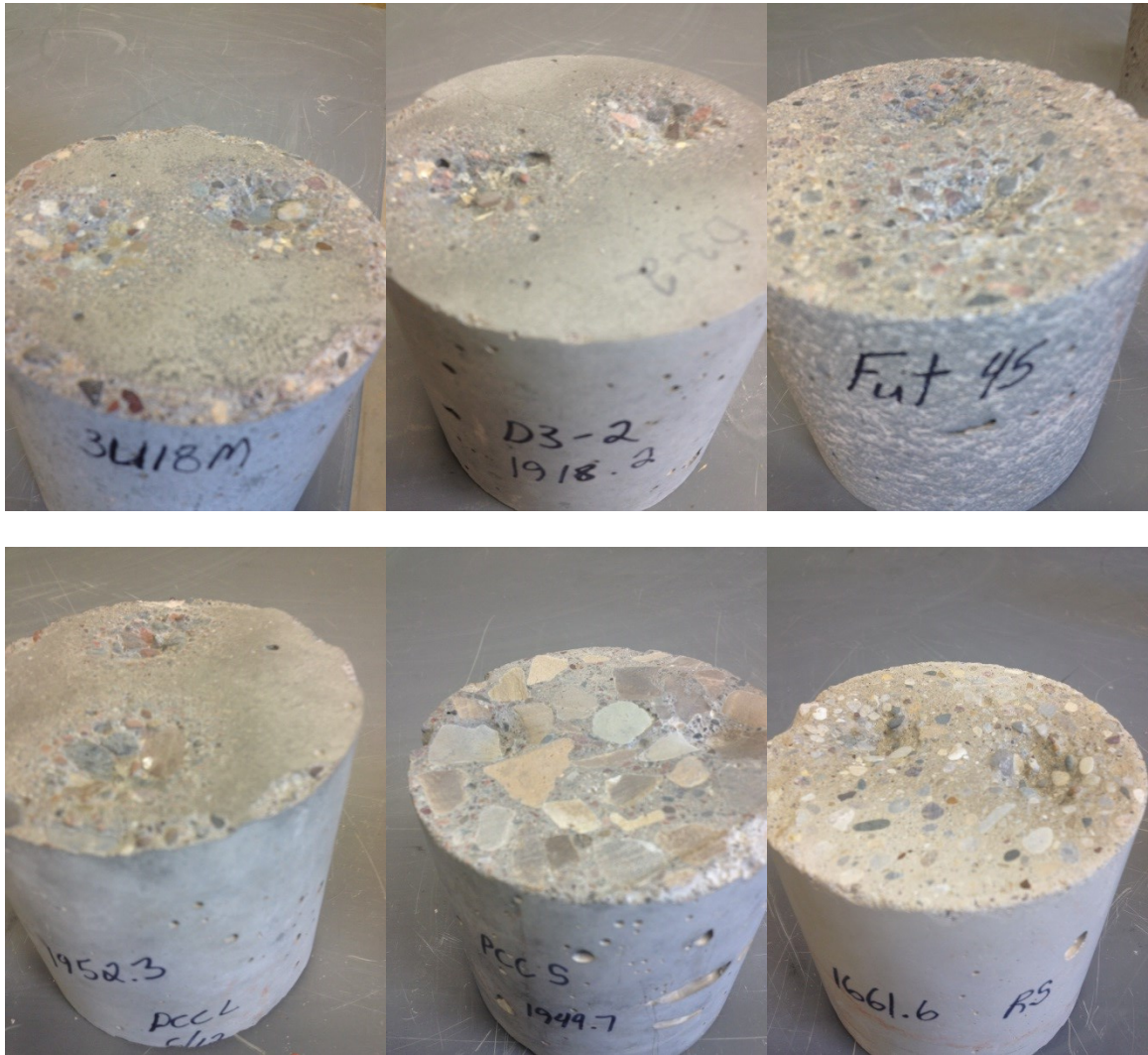
Figure 55: Abrasion test specimens
