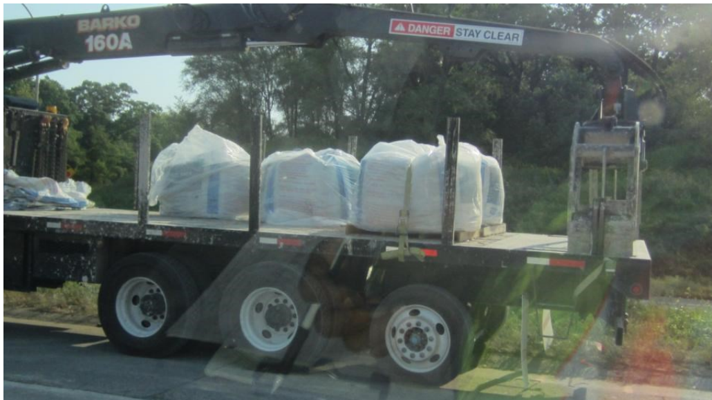
Figure 69: Truck loaded with the pre-bagged rapid set cementitious material
