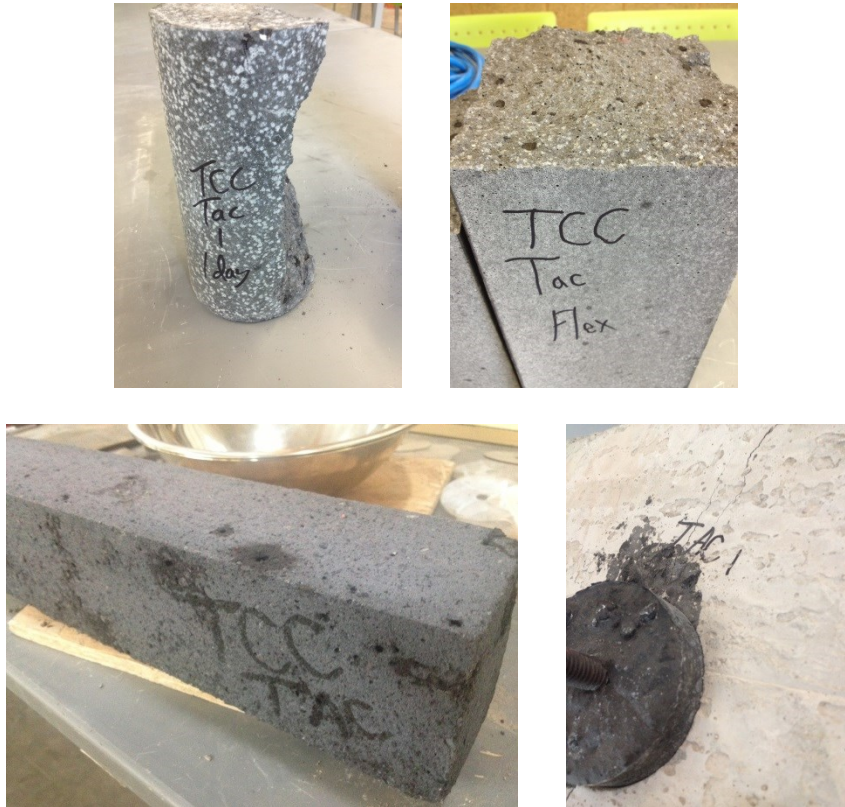
Figure 41: TCC Taconite mix compressive, freeze-thaw, flexural and pull out specimens
