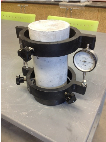
Figure 43: Modulus of Elasticity apparatus with dial gage
