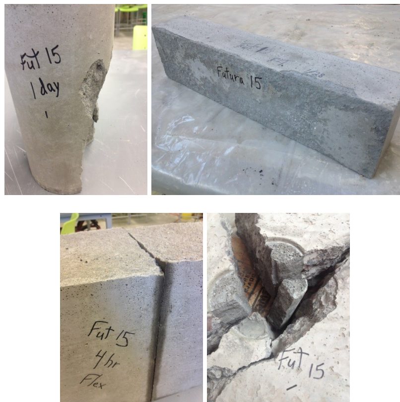
Figure 34: Futura-15 compressive, freeze-thaw, flexural and pull out specimens
