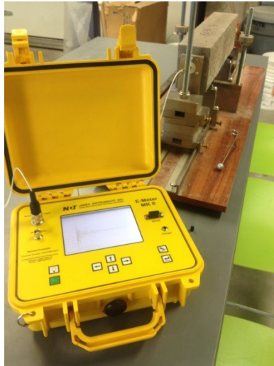
Figure 8: E-meter used to collect frequency data
