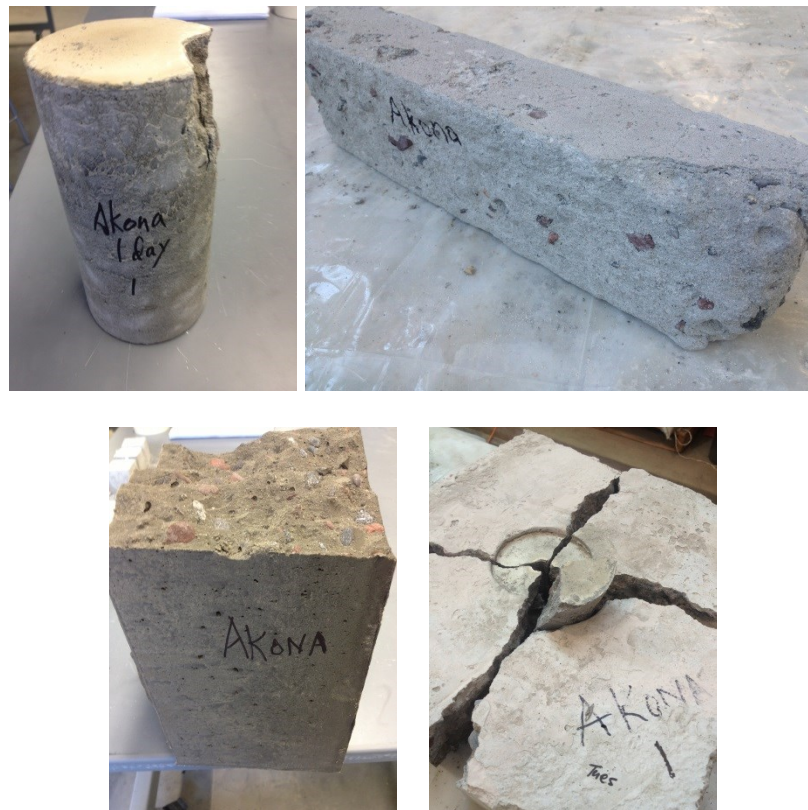
Figure 30: Akona compressive, freeze-thaw, flexural and pull out specimens
