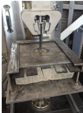
Figure 11: Bond Pullout Testing Fixture in the MTS Machine
