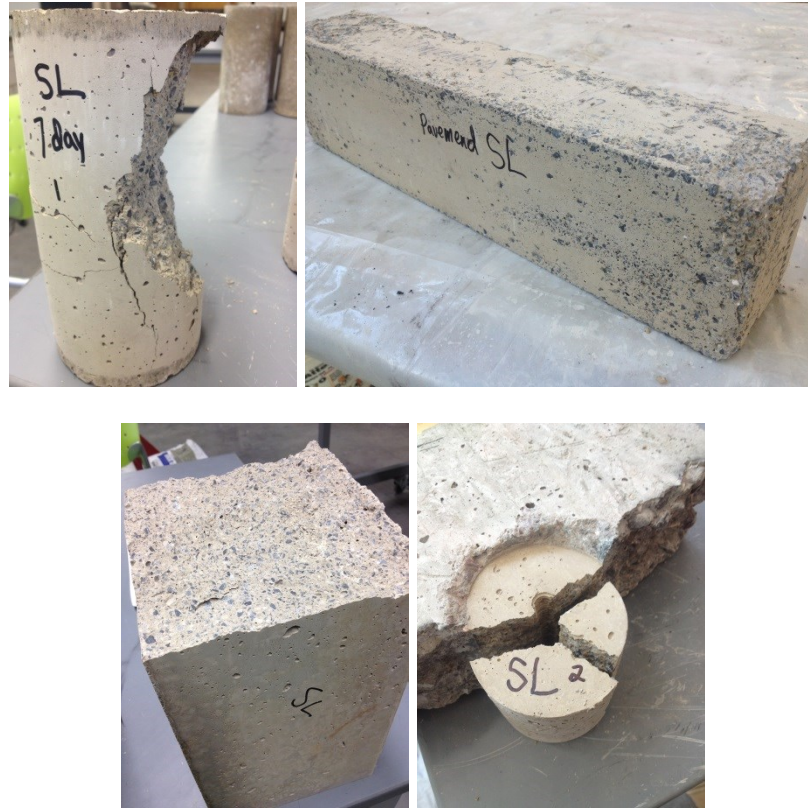
Figure 37: Pavemend SL compressive, freeze-thaw, flexural and pull out specimens
