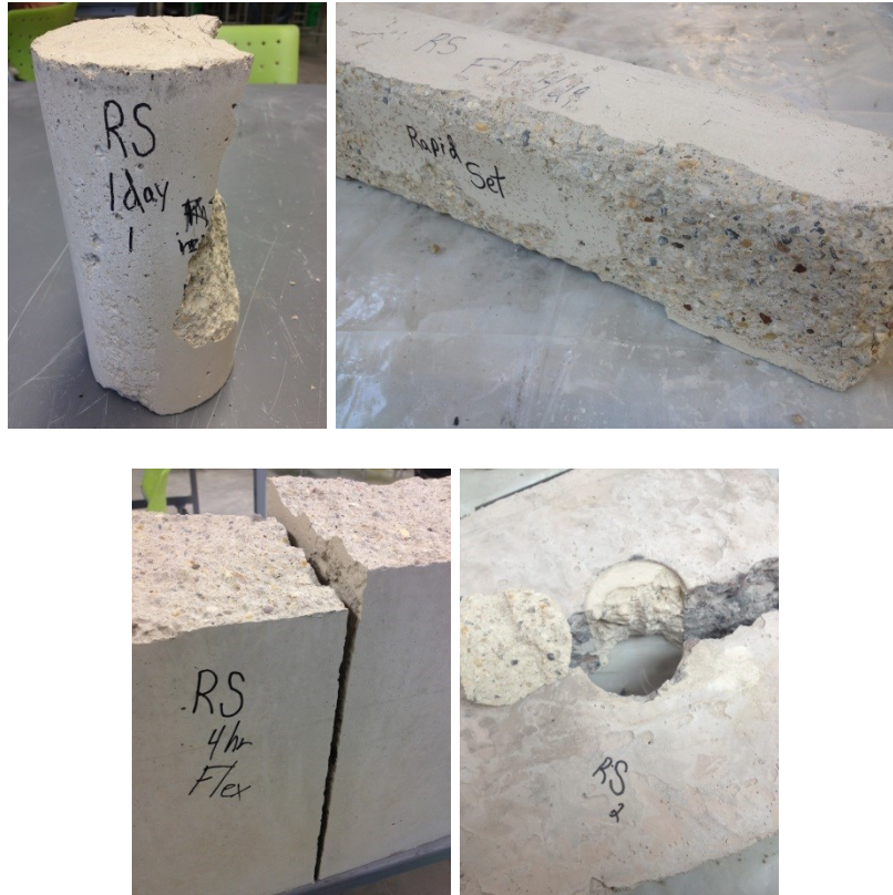
Figure 39: Rapid Set compressive, freeze-thaw, flexural and pull out specimens
