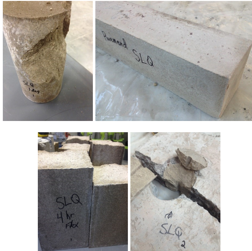
Figure 38: Pavemend SLQ compressive, freeze-thaw, flexural and pull out specimens
