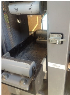
Figure 5: Four-point Bending Test Fixture in Compression Frame
