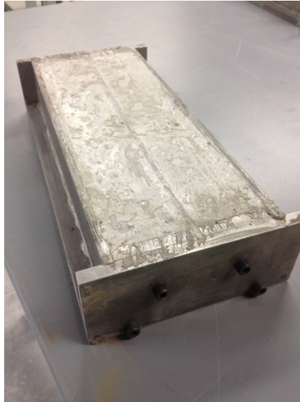
Figure 45: Length change in sulfate specimen mold
