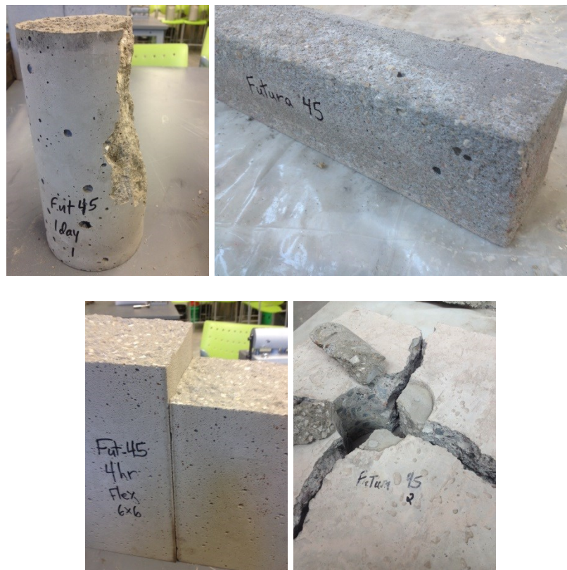
Figure 35: Futura-45 compressive, freeze-thaw, flexural and pull out specimens
