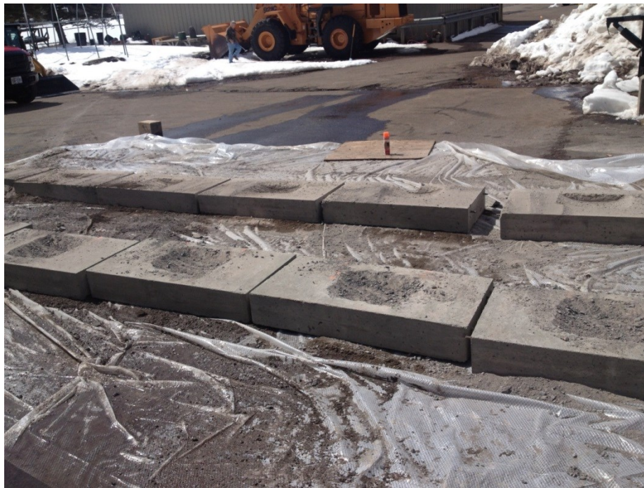
Figure 47: Test slabs for the pop-out bond test
