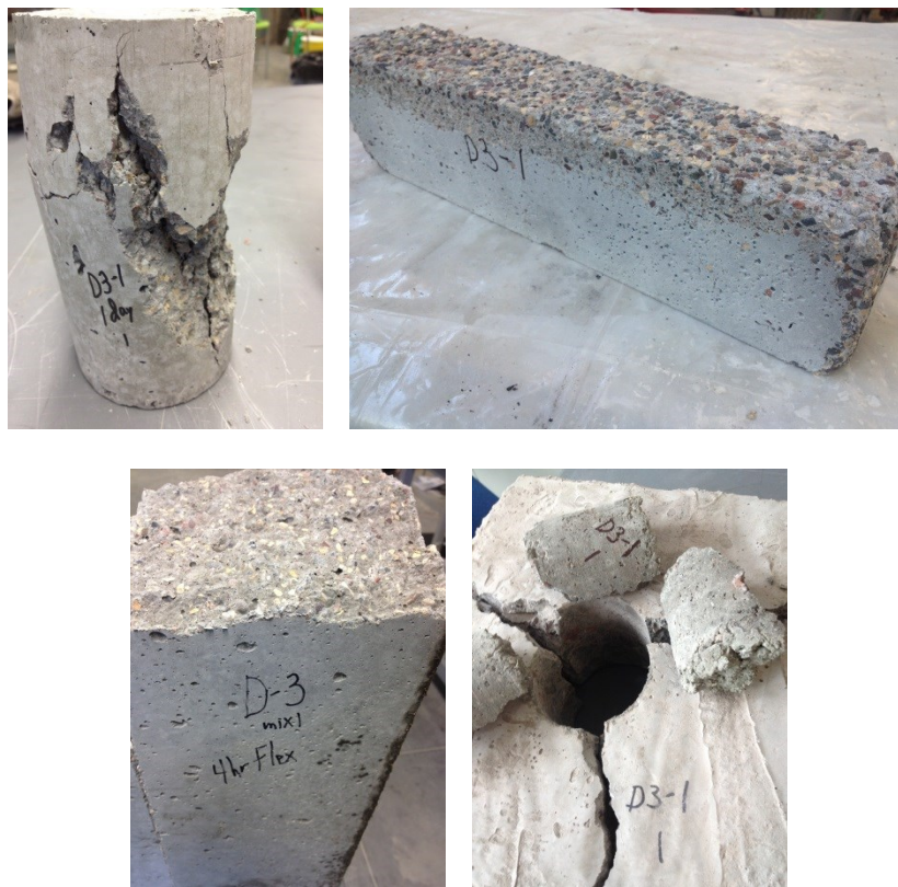
Figure 31: MnDOT District 3 Mix 1 compressive, freeze-thaw, flexural and pull out specimens
