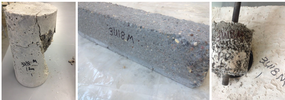
Figure 29: 3U18M compressive, freeze-thaw and pull out specimens
