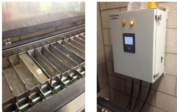
Figure 9: Freeze-Thaw Chamber and Digital Control Box
