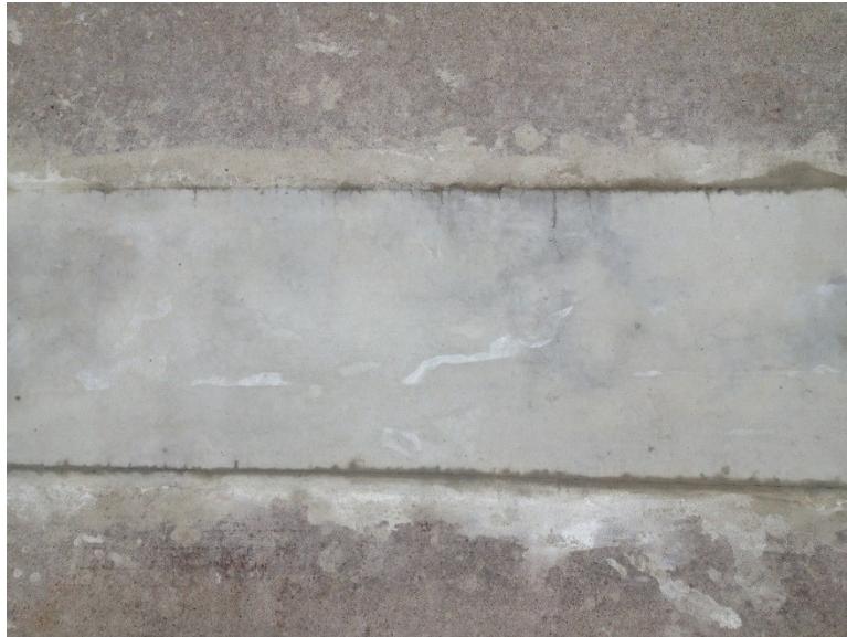
Figure 63: Wetted and covered curing method result
