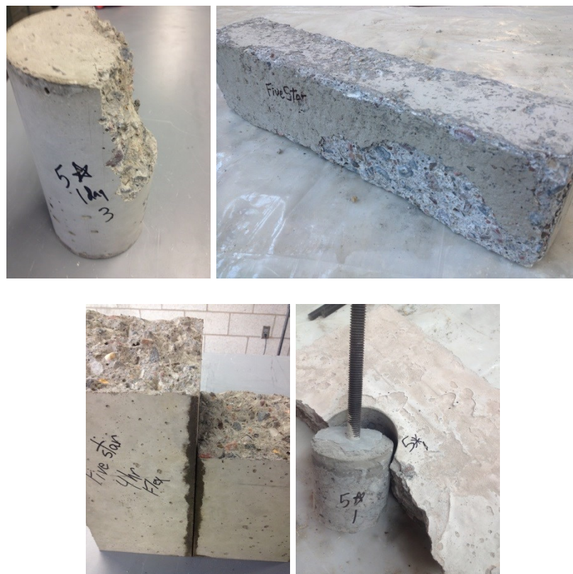
Figure 33: Five Star compressive, freeze-thaw, flexural and pull out specimens
