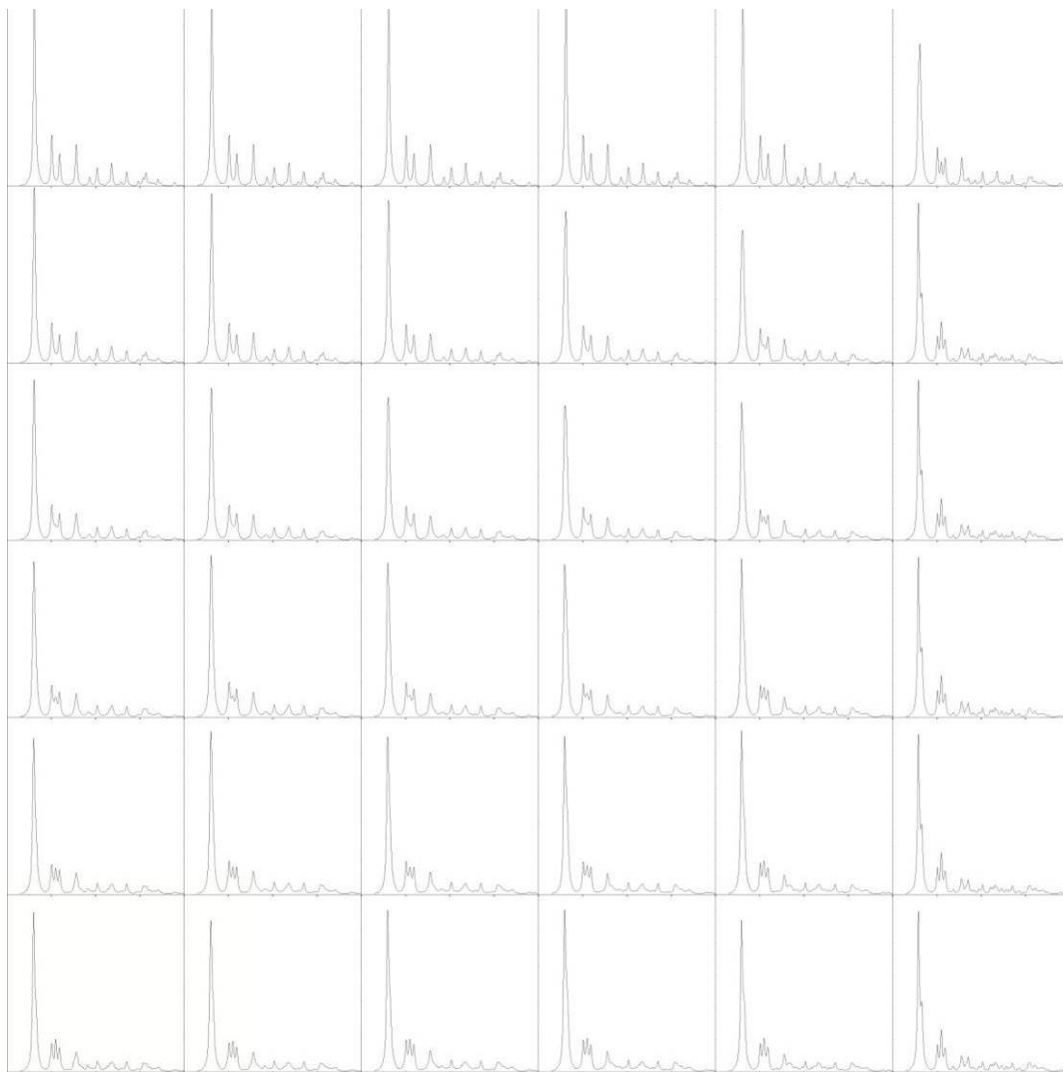
Figure 7-25 Simulated powder XRD patterns of nanoparticles using DIFFaX. The nanoparticle dimensions are: 25 nm wide layers, 15 layers for each particle. The horizontal axis is \alpha_{EE} from 0 to 1 (0.0, 0.2, 0.4, 0.6, 0.8, and 1.0), the vertical axis is \alpha_{FF} from 0 to 1 (0.0, 0.2, 0.4, 0.6, 0.8, and 1.0).
