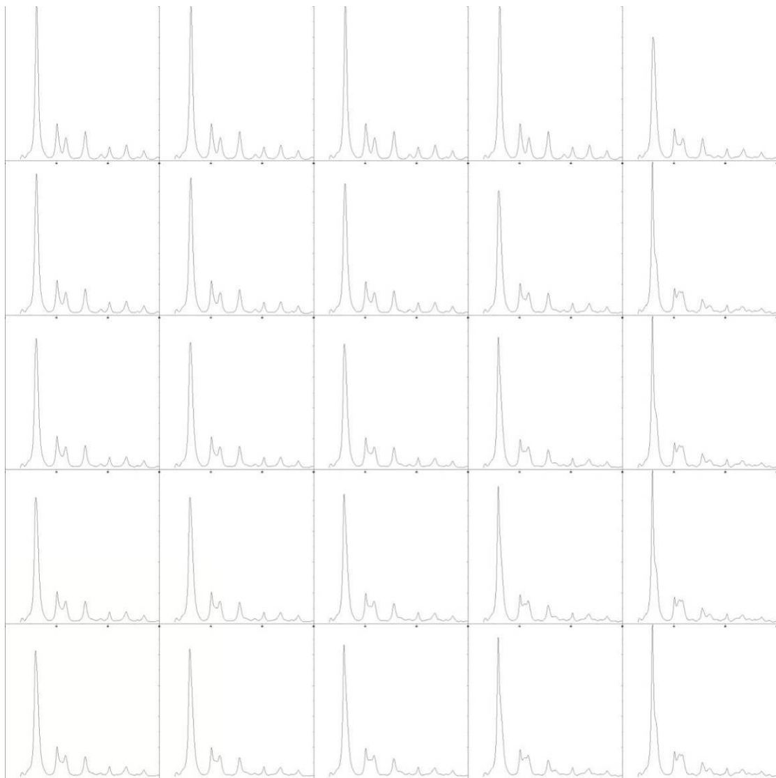
Figure 7-28 Simulated powder XRD patterns of nanoparticles using DIFFaX. The nanoparticle dimensions are: 25 nm wide layers, 10 layers for each particle. The horizontal axis is \alpha_{EE} from 0.80 to 1 (0.80, 0.85, 0.90, 0.95, and 1.0), the vertical axis is \alpha_{FF} from 0.80 to 1 (0.80, 0.85, 0.90, 0.95, and 1.0).
