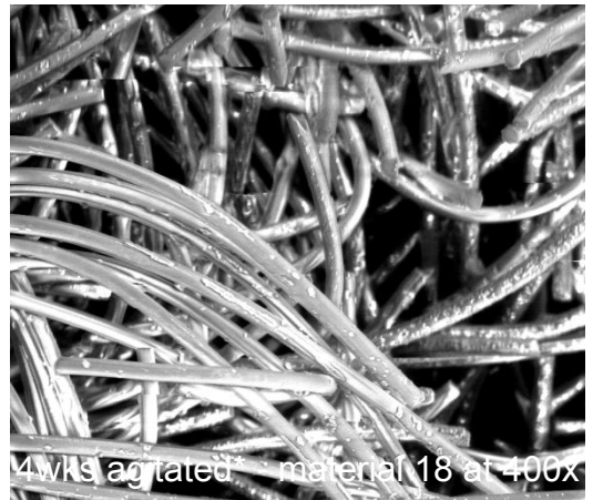
Figure 31: Baseline and 4 weeks agitated SEM images for PGA knit material 18 magnified 100 and 400 times
